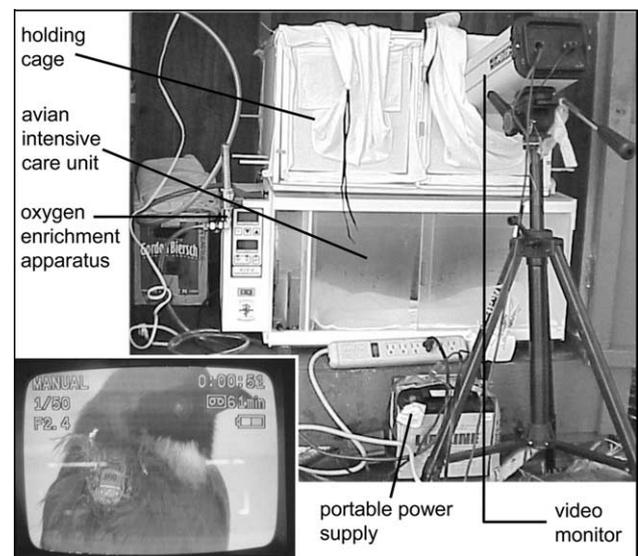
Fig. 3. Equipment set-up for veterinary care and field monitoring of Po’ouli held whilst under captive field conditions. Inset: view through remote TV monitoring system of HR1 Po’ouli individual with radio transmitter attached. Photographs by Maui Forest Bird Recovery Project.
